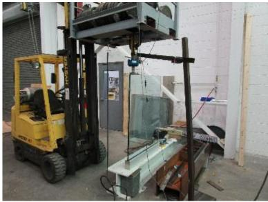
Photo No. 4 Concentrated Load Test at Top Corner of Glass Panel (Vertical)
