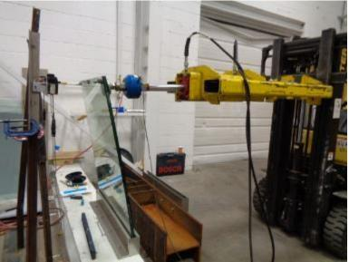
Photo No. 3 Concentrated Load Test at Top Corner of Glass Panel (Applied from Exterior Side)
