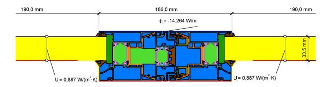
$$U_{_{fAB}} = \frac{\frac{\Phi}{\Delta T} - U_{_{p1}} \cdot b_{_{p1}} - U_{_{p2}} \cdot b_{_{p2}}}{b_{_{f}}} = \frac{\frac{14,264}{20,000} - 0,887 \cdot 0,190 - 0,887 \cdot 0,190}{0,186} = 2,0 \text{ W}/(\text{m}^2 \cdot \text{K})$$
