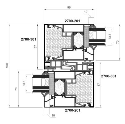
Fig. 3 Cross section test specimen -03\*
