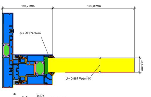
$$U_{r} = \frac{\frac{\Phi}{\Delta T} - U_{p} \cdot b_{p}}{b_{r}} = \frac{\frac{9,274}{20,000} - 0,887 \cdot 0,190}{0,117} = 2,5 \text{ W/(m}^{2} \cdot \text{K)}$$
