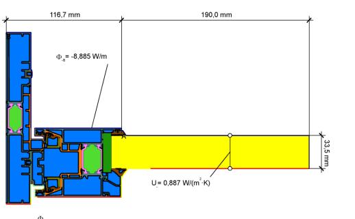
$$U_{fAB} = \frac{\frac{\Phi}{\Delta T} - U_{p} \cdot b_{p}}{b_{c}} = \frac{\frac{8,885}{20,000} - 0,887 \cdot 0,190}{0,117} = 2,4 \text{ W/(m}^{2} \cdot \text{K)}$$
