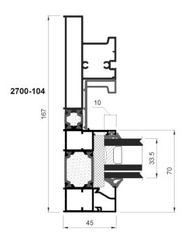
Fig. 5 Cross section test specimen -05\*
