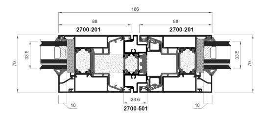
Fig. 4 Cross section test specimen -04\*
