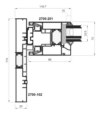
Fig. 8 Cross section test specimen -08\*
