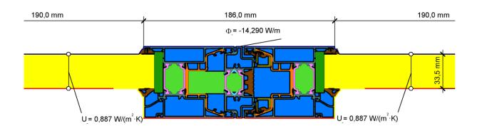
$$U_{_{fAB}} = \frac{\frac{\Phi}{\Delta T} - U_{_{p1}} \cdot b_{_{p1}} - U_{_{p2}} \cdot b_{_{p2}}}{b_{_{f}}} = \frac{\frac{14,290}{20,000} - 0,887 \cdot 0,190 - 0,887 \cdot 0,190}{0,186} = 2,0 \text{ W}/(\text{m}^2 \cdot \text{K})$$
