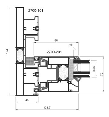
Fig. 1 Cross section test specimen -01\*
