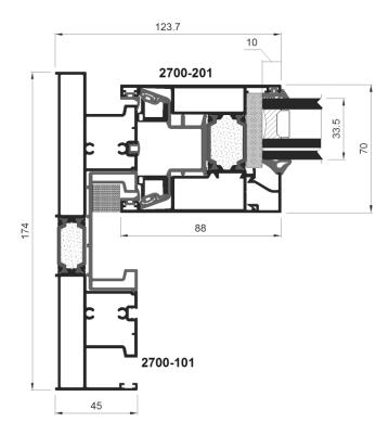
Fig. 2 Cross section test specimen -02\*
