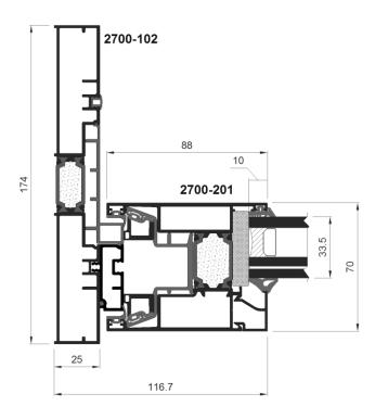
Fig. 7 Cross section test specimen -07\*
