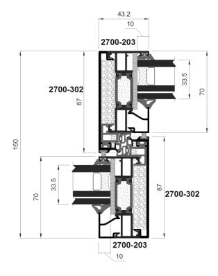
Fig. 6 Cross section test specimen -06\*
