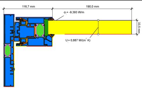
$$U_{r} = \frac{\frac{\Phi}{\Delta T} - U_{p} \cdot b_{p}}{b_{r}} = \frac{\frac{9,393}{20,000} - 0,887 \cdot 0,190}{0,117} = 2,6 \text{ W/(m}^{2} \cdot \text{K)}$$
