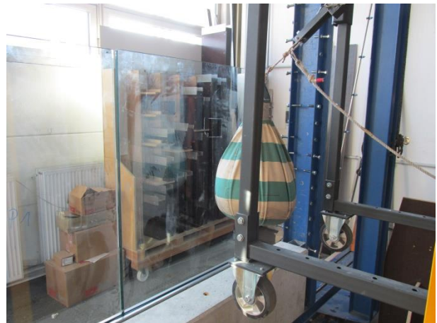
Picture 20 Pendulum test - P2 before testing
