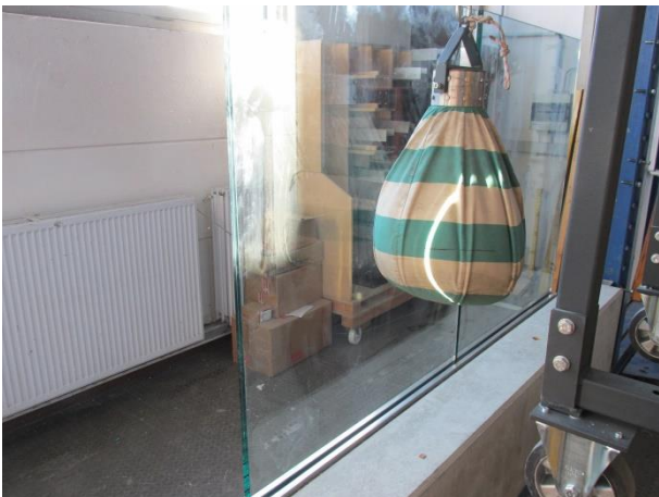
Picture 19 Pendulum test - P1 after testing
