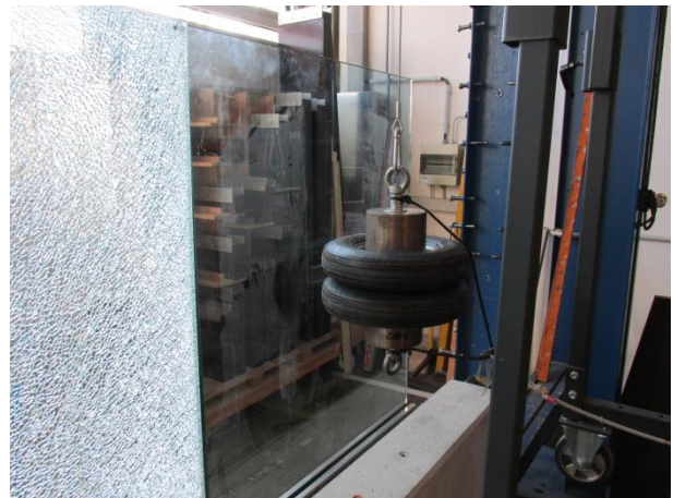
Picture 24 Pendulum test - P1 after testing with twin tyres
