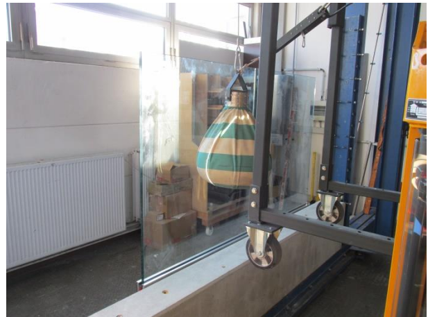
Picture 18 Pendulum test - P1 before testing
