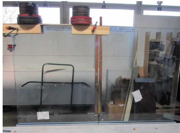
Picture 6 Static inward test - Test with 0.2 kN/m
