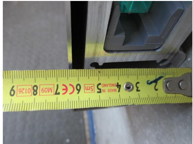
Picture 10 Pendulum test - dimension of Aluminium Profile
