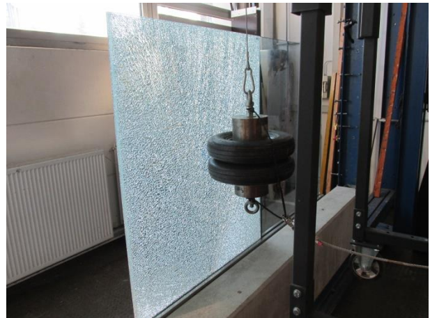
Picture 24 Pendulum test - P1 after testing with twin tyres
