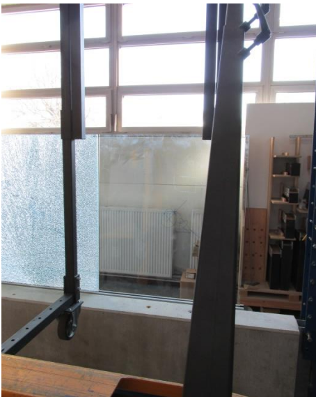
Picture 25 Pendulum test - P2 before testing with twin tyres
