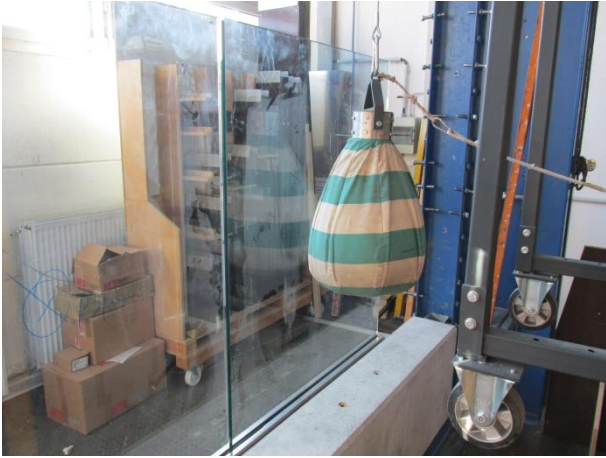
Picture 21 Pendulum test - P2 after testing
