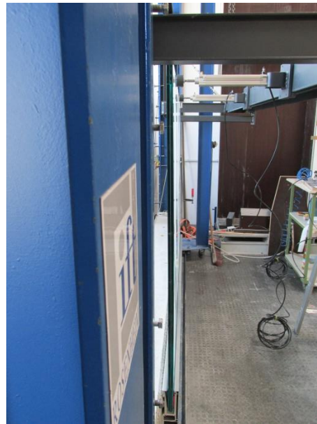
Picture 6 Static inward test - Test with 0.2 kN/m
