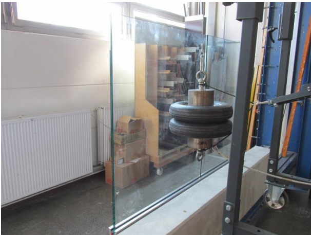
Picture 23 Pendulum test - P1 before testing with twin tyres
