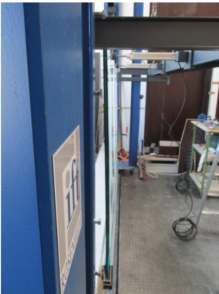
Picture 7 Static inward test - Test with 0.4 kN/m
