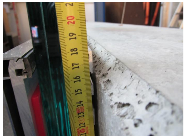
Picture 14 Pendulum test - dimension of Aluminium Profile
