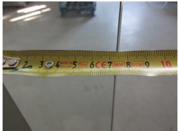
Picture 10 Sideways overhang of the glass
