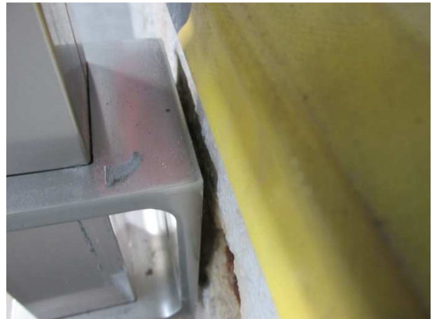
Picture 14 Screw pull-out after the first pendulum impact
