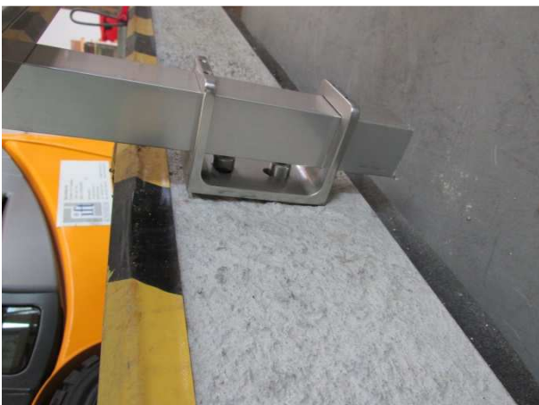
Picture 15 Screw pull-out after the second pendulum impact
