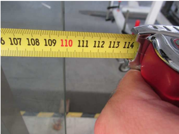
Picture 3 Width of laminated glass
