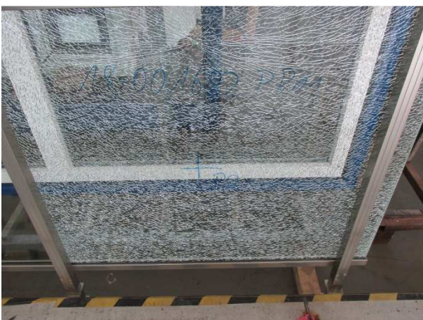
Picture 17 Breakage typical for TSG
