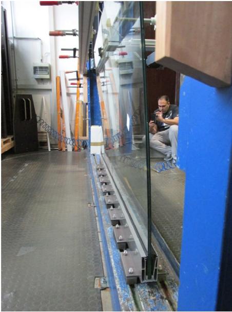
Picture 7 Deformation under load vom inside to outside
