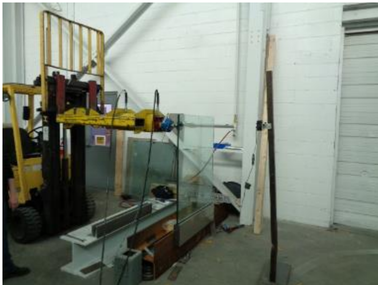
Photo No. 2 Concentrated Load at Top Corner of Glass Panel
